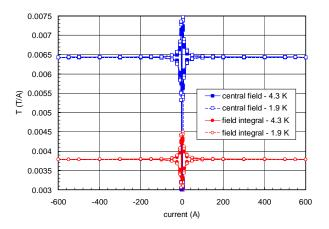
Figure 3: Transfer functions of the inner dipole. Both central field and field integrals at 4.3K and 1.9 K are shown.
