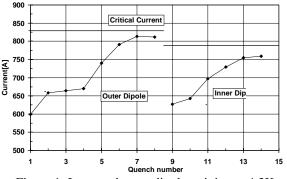
Figure 1: Inner and outer dipole training at 4.3K
