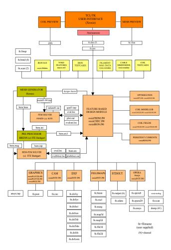
Figure 1: Structure of the ROXIE program featuring a TCL/TK user interface (top), and various interfaces to CAD-CAM (bottom). The interfacing to the finite-element packages is done by means of file transfer.
