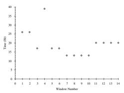
Figure 4: RFQ vacuum window conditioning time.
