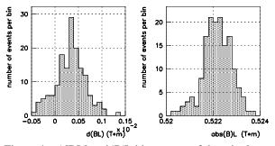
Figure 4 :  $\Delta[BL]$  and |B|L histograms of the wigglers
