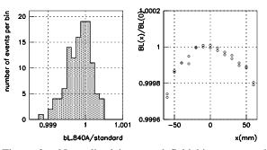
Figure 2 : Normalized integrated field histogram and an example of its transverse distribution for HER  $B_{arc}$
