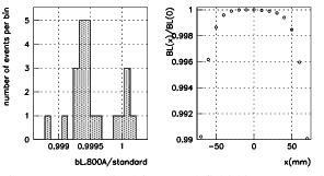
Figure 3 : Normalized integrated field histogram and an example of its transverse distribution for LER  $B_{lc}$
