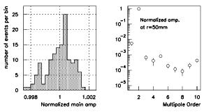
Figure 6: Normalized integrated field gradient (left) and normalized multipole amplitudes plotted as a function of multipole order (right) for HER QA.
