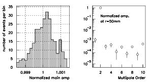
Figure 5 : Normalized integrated field gradient (left) and normalized multipole amplitudes plotted as a function of multipole order (right) for LER Q<sub>arc</sub>.
