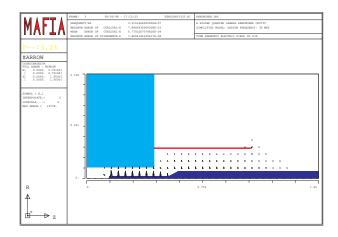
Figure 2: An optimized 2D (rz geometry) MAFIA model for the 35 MHz re-buncher RF cavity. The dimensions of the cavity shown here may not be the final, but close to. The arrows shown in the cavity are the electric field strength.
