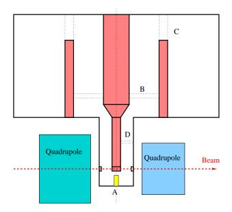
Figure 1: Schematic layout (not to scale) of the 35 MHz rebuncher RF cavity for ISAC at TRIUMF. Dotted lines and notations of **A**, **B**, **C** and **D** are reserved for possible locations of a tuner, a disk RF window, a tubular RF window and supporting ceramic rods, respectively.
