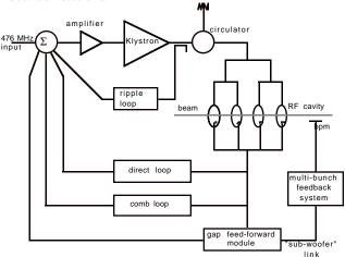
Figure 4 Low-level RF system block diagram
