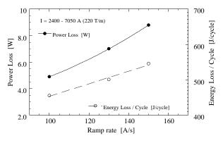
Fig. 5. AC loss measured as function of the ramp rate.
