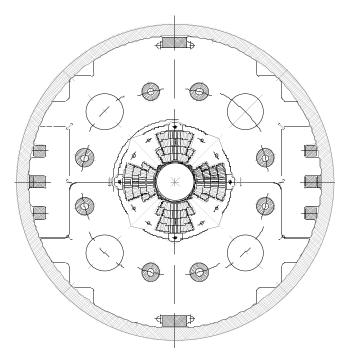
Fig. 1: Cross section of the first low- $\beta$  quadrupole model.
