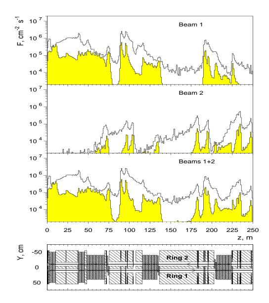
Figure 2: Hadron flux density around the beam lines. Clear histograms - the case without shielding, grey histograms - the case with shielding. The z-range covers a half of the staight section. Beam enters at z=0, where the primary collimators are located. F(z) in z=[250,500] for beam 2 is similar to F(z) for beam 1 left-right reflected.
