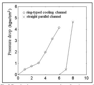
Fig. 3 Cumulated water pressure drop for ring-typed cooling channels(1-6) and straight parallel ones(7-8)
