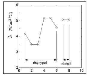
Fig. 2 Surface heat transfer coefficient *h* for ring-typed cooling channels(1-6) and straight parallel ones(7-8)
