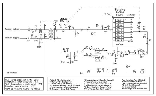
Fig. 4 Schematic drawing of the water cooling system for the passive Landau cavity at SRRC.
