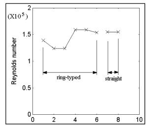
Fig. 1 Reynolds number for ring-typed cooling channels (1-6) and straight parallel channels (7-8)
