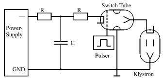
Figure 1: Basic Circuitry of a Hard Tube Pulser
