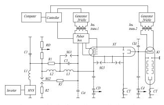
Figure 2: Circuit of a 600 kV Hard Tube Pulser HVS-high voltage source; Kl-klystron; ST-switch tube; CT-current transformer; RD-resistive divider; CD-pulse divider;  $L_1$ -protection choke;  $C_1$ ,  $C_3$ ,  $L_2$ ,  $L_3$ ,  $R_1$ - elements of PFN;  $C_{st}$ ,  $C_{kl}$ -spurious capacitance;  $R_2$ ,  $R_3$ limiting resistors; SG1, SG2, SG3-protection spark gaps.
