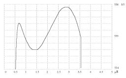
b: Pulse Flat-top on Klystron (200 V/div)
