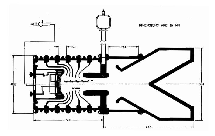
Figure 4: Design of the proposed Switch Tube.
