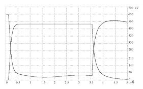
a: Pulse Voltage on Klystron and Switch Tube (70 kV/div)
