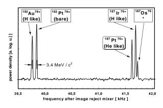
Figure 2: Zoomed part of a Schottky mass spectrum of electron cooled Au-fragments in the ESR. Additional lines are resolved from nearly 60 peaks seen in the original 100 kHzspectrum. The published mass value for the <sup>187</sup>Pt-nucleus could be improved essentially with respect to absolute value and relative error.
