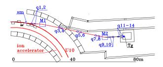
Figure 2. Layout of final beam transport channel for TWAC.
