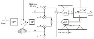
Figure 3. The bunch-by-bunch phase measurement circuit. The I/Q components of the response of the Bessel filter (Q=10) are demodulated with the components of the reference signal at 28 MHz. Digital rectangular-to-polar conversion supplies the phase and magnitude.
