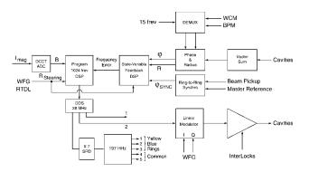
Figure 1. Block diagram of beam control system. Two DSPs calculate the frequency program, and the feedback algorithms. Each ring has two 28 MHz cavities and five 197 MHz cavities. A <u>Step Recovery D</u>iode generates the 197 MHz from the 28 MHz. Standard RHIC <u>Wave Form Generators update at 720 Hz</u>.
