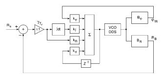
Figure 2. State variable feedback.  $B_R$  and  $B_{\phi}$  are beam transfer functions. There are four states, including an integral of the radial error and a delay compensator. At transition the sign of the radial feedback is changed.
