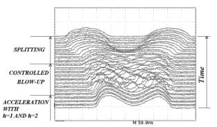
Figure 2 : Splitting and blow-up at the end of acceleration in the PSB  $(3x10^{12} \text{ protons})$ .
