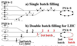
Figure 1 : (a) PS single and (b) double batch filling schemes.
