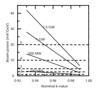
Figure 1: Required power of proton beam versus reactor multiplying coefficient. Dashed line means: 1- PSI - 1.8 mA, 0.59 GeV, 2- PSI - 5.0 mA, 3 - DC-2.5 mA, 1 GeV/nucl., 4- DC - 5.0 mA, 5 - DC -10.0 mA.
