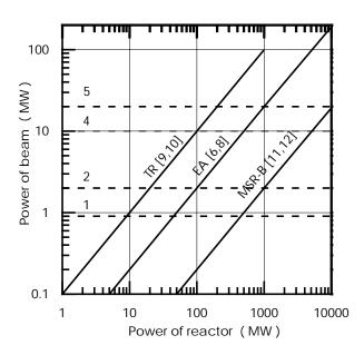
Figure 2: Required power of proton beam versus reactor power at  $k_{eff}$ =0.95. Dashed lines mean the same as in Fig.1.
