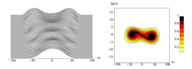
Figure 3: Quasi-adiabatic bunch splitting at 3.5 GeV/c.
