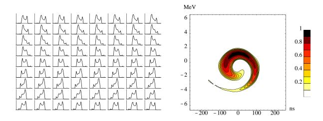
Figure 2: Measured profiles and reconstructed contour plot of a phase-modulated bunch at 1 GeV.
