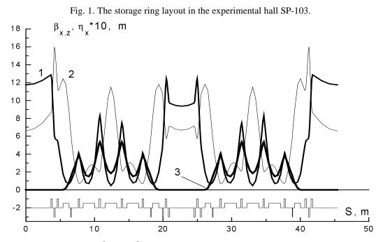
Fig. 2. Lattice functions  $\beta_x - (1)$ ,  $\beta_z - (2)$  and  $\eta_x \cdot 10 - (3)$  the proposed ring in SLS operating mode.
