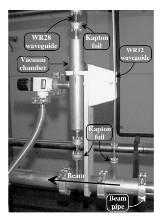
Figure 2: Beam pipe-waveguide coupling as installed in the CTF drive linac.
