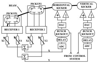
Figure 1: Transverse feedback system concept.
