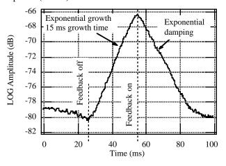
Figure 6: Typical growth/damping rate measurement (lower vertical sideband of  $1f_0$ ,  $I_{av} = 80$  mA).
