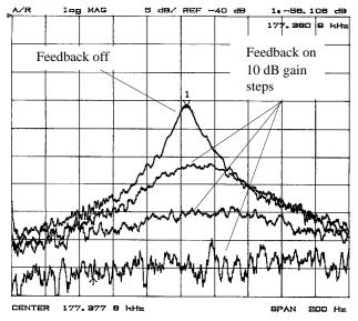
Figure 5: Feedback effect on driven sideband (lower horizontal of 2f<sub>0</sub>) for several different gains.
