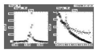
Figure 3: The FFT spectrum of the real (dots) and virtual (boxes) BPM. On the left the central part of the spectrum is shown, on the right a detail from the upper tail
