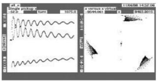
Figure 13: Beam trapped on a third order resonance
