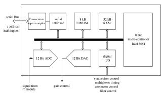
Figure 2: Digital part of the BPM electronics
