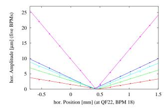
Figure 3: Example of the determination of the BPM zero position using quadrupole current modulation and a local beam bump
