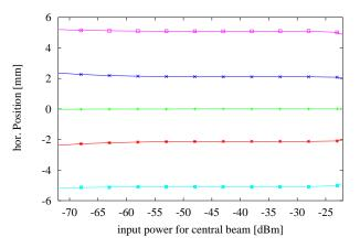
Figure 5: Position stability as a function of the input power for 0 mm,  $\pm$  2 mm, and  $\pm$  5 mm
