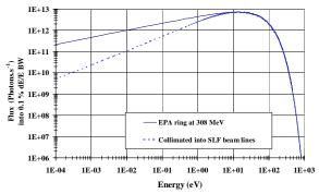
Figure 4: Photon flux in SLF lines (308 MeV, 115 mA).
