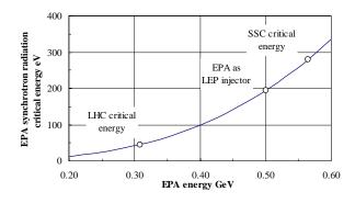
Figure 3: Critical photon energies versus EPA beam energies.
