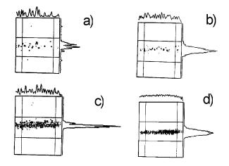
Fig.2 Image of SR beam and profiles on one TV frame for different storage ring beam current. a ) I= 2.5 mA, b) I=5 mA, c) I=10 mA, d) I=25 mA
