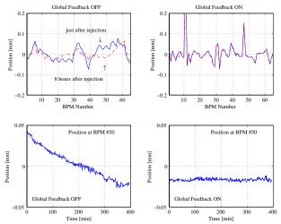
Figure 2: Change in COD without feedback (upper left) and with feedback (upper right) in eight hours. The peaks at the BPM#11 and #47 are due to the trouble of the electrodes. Lower left and right graph show the position change at BPM#50.
