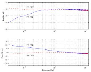
Figure 5: Frequency response of the feedback loop. In this case, -3dB point is about 0.3Hz.
