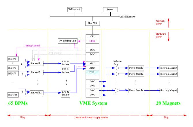
Figure 1: Block diagram of the global feedback system. Station#1-#12 contain multiplexers and superheterodyne detectors. (LPF:Low Pass Filter, ATT: Attenuator, SW Control: Switch control)
