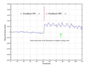
Figure 4: Beam motion at BPM#50.
