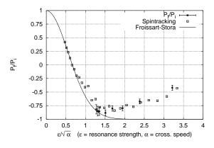
Figure 4: Change in polarization level due to crossing of the imperfection resonance at 1.76 GeV.
