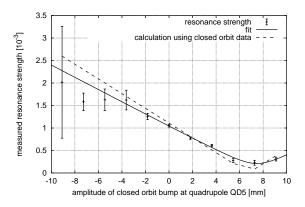
Figure 3: Harmonic correction of the imperfection resonance at 1.32 GeV using a closed orbit bump.
