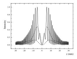
Figure 3: - component of the interfering edge radiation (solid line) and for two edges singly (dashed lines) vs. z.
