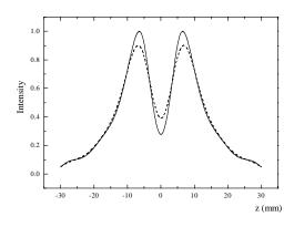
Figure 6: - component of the interfering edge radiation vs. z for the beam with real emittance (solid line) and for the double emittance magnitude (dashed line).
