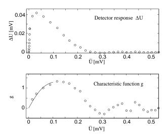
Figure 3: Upper graph: The detector response  $\Delta U$  as a function of  $\overline{U}$ . Lower graph: The characteristic function g, as defined by Equation (3), plotted versus  $\overline{U}$ . The solid line shows an extrapolation of g for small  $\overline{U}$ .
