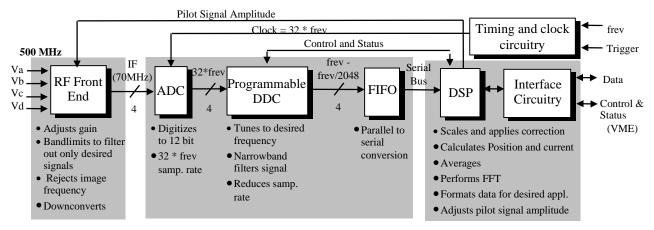
Figure 1: Block diagram of the digital BPM electronics for SLS
