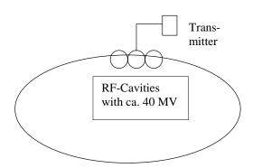
Fig. 4: The basic idea how to obtain a good energy resolution in a muon collider by using the longitudinal polarization. The finite momentum compaction factor together with the cavities let particles with an energy deviation oscillate around the central energy.
