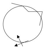
Fig. 3: Situation as in fig. 2 with the only difference that the storage ring is a strong focusing machine. The revolution frequency of the energy deviating particle schematically sketched by the zig-zag line (symbolizing the focusing by quadrupoles) is almost energy independent and the polarization decays more and more from revolution to revolution
