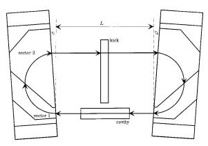
Figure 3: Simplified model of the racetrack microtron.
