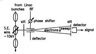
Figure 4: Basic layout of a Bunch Length Detector (BLD, according to [9]).
