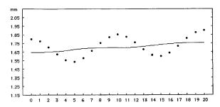
Figure 5: Schematic presentation of beam size evolution over 20 turns, as seen by a screen (OTR or scintillator) or a SEM-grid (from [17]).
