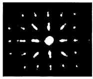
Figure 3: The particles passing through the holes of a pepper-pot and a drift space form elongated images on a scintillator screen (from [4]).
