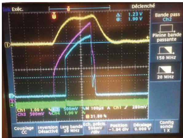
Figure 5: First accelerated H + beam by IPHI RFQ.
