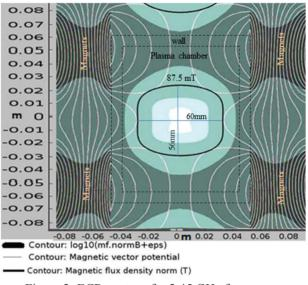
Figure 2: ECR contour for 2.45 GHz frequency.
