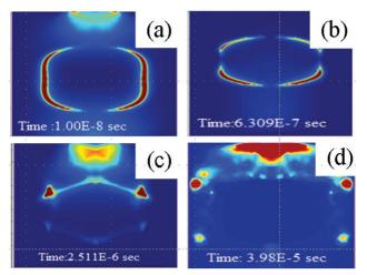
Figure 9: Maximum Power density at different time instants. (a)  $6.6 \times 10^4$  W/m<sup>3</sup>, (b)  $1.43 \times 10^7$  W/m<sup>3</sup>, (c)  $3.12 \times 10^6$  W/m<sup>3</sup> and (d) $1.67 \times 10^7$  W/m<sup>3</sup> at pressure  $10^{-2}$  mbar, 50 W power.
