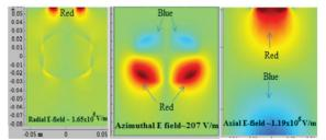
Figure 4: E-field distribution in plasma for 50W total absorbed power and 10<sup>-2</sup>mbar pressure.
