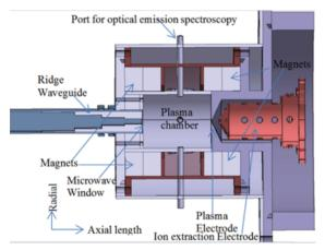
Figure 1: Cut section of negative hydrogen PMECRIS.
