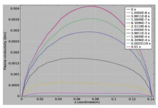
Figure 8: Variation of plasma conductivity with axial distance for different time, without magnets.
