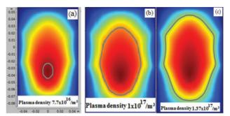
Figure 5: Plasma density contours at different pressures (a)  $2 \times 10^{-3}$  mbar, (b)  $3 \times 10^{-3}$  mbar, (c)  $5 \times 10^{-3}$  mbar. Thick grey line represents critical plasma density of  $7.4 \times 10^{16}$  /m<sup>3</sup>. Total plasma absorbed power is fixed at 50 W.
