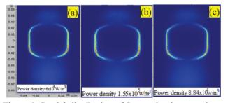
Figure.6: Spatial distribution of Power density at various pressures (a)  $2 \times 10^{-3}$  mbar, (b)  $3 \times 10^{-3}$  mbar and (c)  $5 \times 10^{-3}$  mbar and at constant absorbed power of 50 W.
