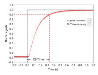
Figure 1: Principle of the traditional  $\tau_{CB}$  measurement. The dashed lines are the references of the pulse start (black) and 90% level of the Rb<sup>20+</sup> beam intensity (red).
