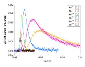
Figure 4: Rb<sup>4+</sup>, Rb<sup>8+</sup>, Rb<sup>10+</sup> Rb<sup>13+</sup>, Rb<sup>17+</sup> and Rb<sup>19+</sup> beam intensity responses to a 2.5 ms injection pulse.
