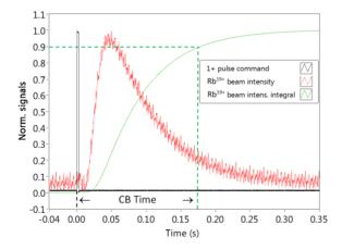
Figure 2: Rb19+ response to a 2.5 ms injected pulse and the corresponding integral function. The dashed lines are the references of the pulse start (black) and 90% level of the Rb19+ integral function (green).
