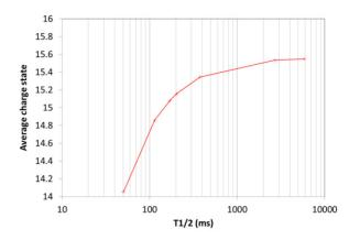
Figure 9: Evolution of the average ion beam charge state as a function of the half-life.
