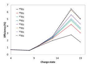
Figure 8: Rb isotope efficiencies as a function of the charge state.
