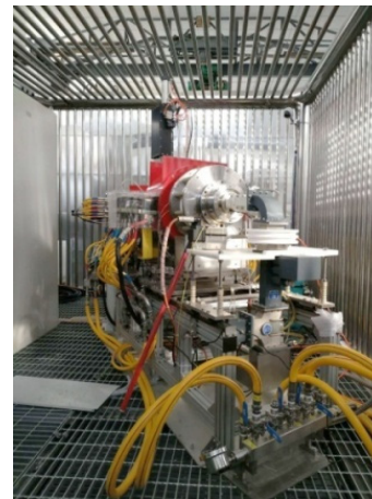
Figure 4: Front view of the 400kV high voltage accelerator
