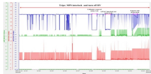
Figure 3: Operation log of the ion source with the time of 240 hours
