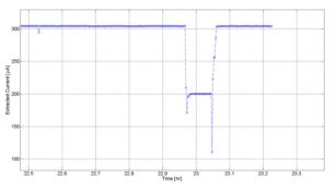
Figure 3. Two step behavior of the current. After the He flow recovers the plasma may stay in a different state leading to a lower source current until it will recover to previous current value.
