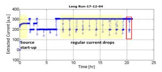
Figure 2. Regular current drops observed in Source 2 [4]. The red rectangle is showing the area presented on the next picture (Fig. 3).
