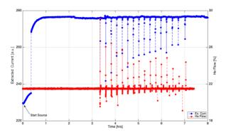
Figure 4. Current drop correlated with support gas flow oscilations
