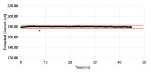
Figure 5. Beam stability after the solving the unstable gas injection.
