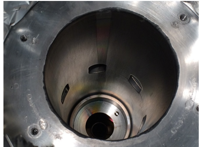
Figure 3: The ANL ECRCB plasma chamber after coating with ultra-high purity aluminum. Note the shadow at the top of the chamber caused by the high current lead which shows the uncoated surface. The aluminum disk at the injection side also still shows the plasma loss lines demonstrating the limitations of the evaporation coating technique.
