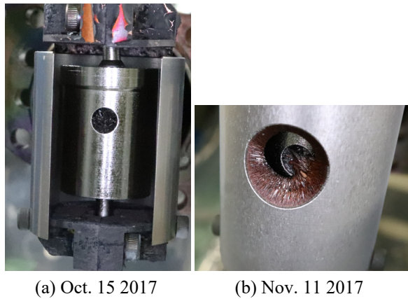
Figure 5: Blockage of the vapor-ejection hole of crucibles.
