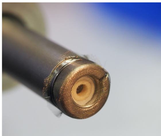
Figure 3: Microwave shielding grid at the oven orifice.
