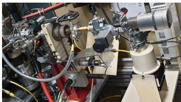
Figure 4: MIVOC process is connected at ECR4 ion source.
