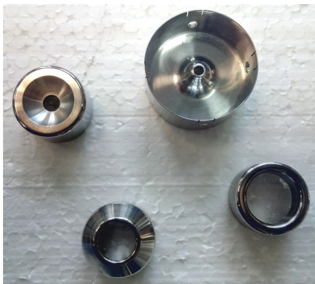
Figure 7: A photograph of spherical plasma electrode and a set of puller electrodes.
