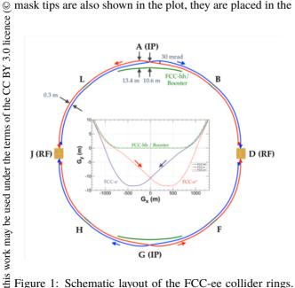
Figure 1: Schematic layout of the FCC-ee collider rings. The green line indicates the beamline of the FCC-ee booster and hadron collider FCC-hh. The plot in the middle shows the two beams trajectories at the IP.
