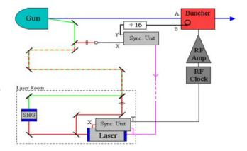
Figure 4: Local and remote synchronisation layouts.
