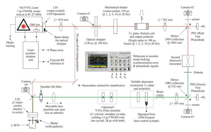
Figure 2: Schematic showing the layout of the optical system for the ERLP photoinjector drive laser.
