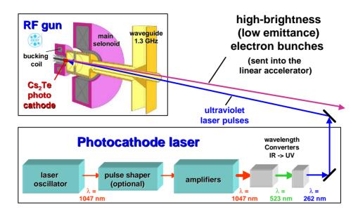
Figure 1: General setup of a photoinjector (picture of the gun by courtesy of K. Floettmann, DESY Hamburg)
