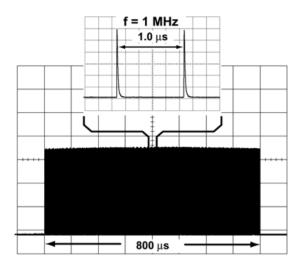
Figure 3: Output pulse train of the Nd:YLF drive laser
