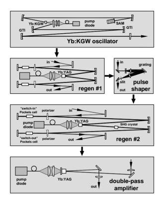
Figure 5: Scheme of the experimental Yb:YAG laser-driver laser under development at the MBI
