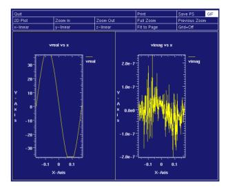
Fig. 5: Integrated accelerating voltage across the cavity. Note the flat tops within beam pipes which are desired for beam acceleration.
