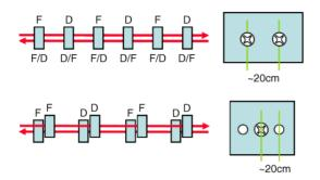
Fig. 7: Conceptual optics layout with dual-axis quadrupoles.
