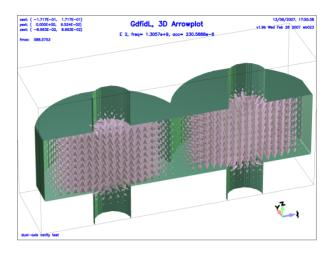
Fig. 1: A conceptual dual-axis single-cell cavity.
