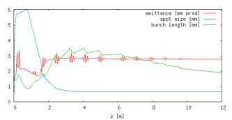
Figure 6. Evolution of the rms values of the normalised transverse emittance, transverse spot size and bunch length along the HACL injection line.
