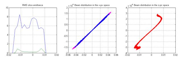
Figure 8. Transverse rms slice emittance (left panel), projected transverse emittance (central panel) and longitudinal emittance (right panel) at the exit of the IR-FEL injector as calculated with the ASTRA code.
