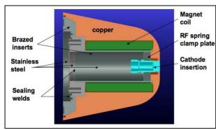
Figure 2: Gun nose assembly schematic.
