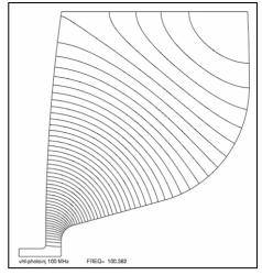
Figure 9: 100MHz cavity geometry.
