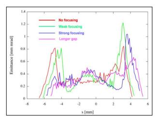
Figure 7: Variation of slice emittance for differing gap geometry. Bunch charge is 0.5nC.
