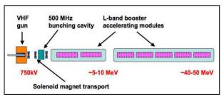
Figure 3: APEX photoinjector beamline.
