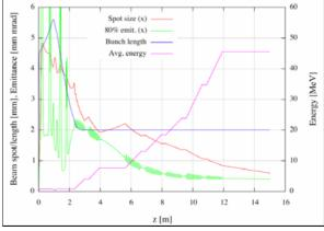
Figure 4: Evolution of beam quality in the photoinjector.
