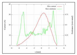
Figure 5: Slice current and emittance at the photoinjector exit (z=15m).
