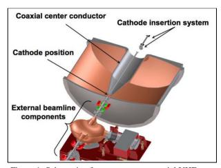
Figure 1: Schematic of a quarter-wave coaxial VHF gun.
