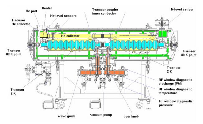
Figure 1: The ELBE linac module for cw operation
