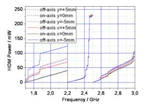
Figure 6: Total damped power of HOM at typical ELBE beam parmeters (  $20 \text{ MeV}, 240 \mu \text{A}$ )
