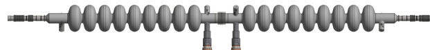
Figure 2: CAD Model of the MESA cavity string. In the bottom center the two HF power couplers can be seen, the four other visible ports (bottom left and right, top center) are the HOM couplers.
