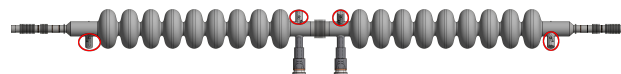
Figure 2: CAD Model of the MESA cavity string. In the bottom center the two HF power couplers can be seen, the four other ports (red circles) are the HOM couplers.
