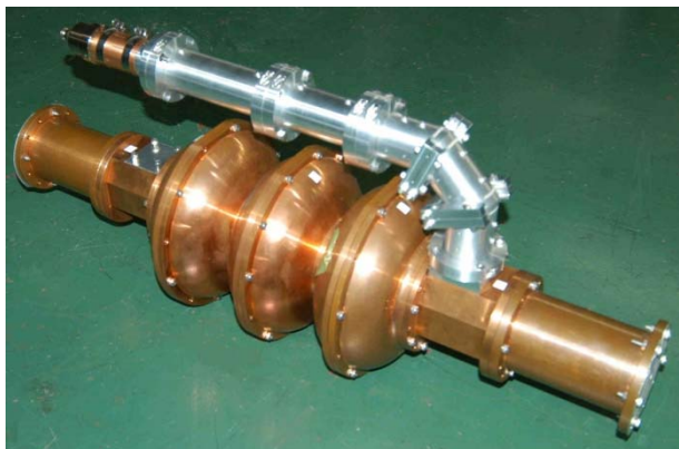
Figure 8: Bent CSWG HOM coupler of bending angle of 45 degrees installed to TESLA type cavity model.
