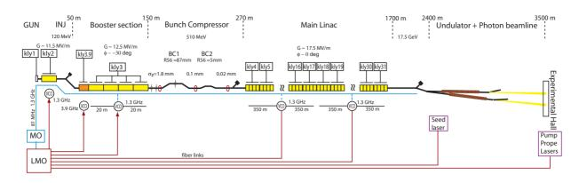
Figure 2: Layout of a 4th generation light source.
