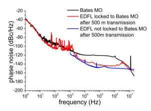
Figure 8: Single sideband phase noise of the Bates Reference Oscillator, the EDFL locked to the reference after transmission through the link and the free running EDFL.
