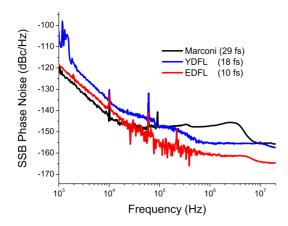
Figure 5: Single-sideband phase noise spectral density for the EDFL, YDFL, and a Marconi 2041 signal generator.
