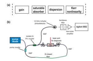
Figure 3: (a) The four effects governing spulse shaping in mode-locked lasers. (b) Schematic of the experimental setup: SMF, single-mode fiber.
